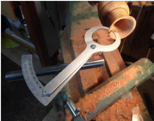
Figure 12. Turn vase lip and establish the wall thickness. Continue hollowing from top to bottom stopping often to measure wall thickness.
