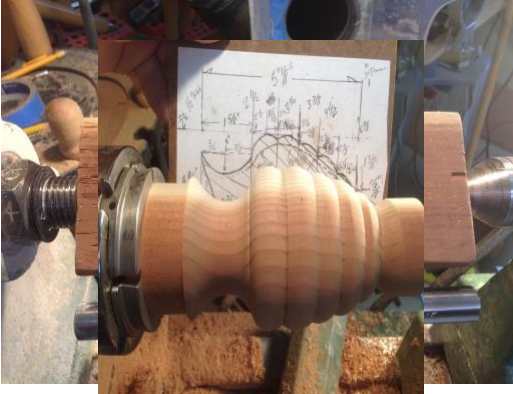
Figure 4. Start with a blank larger than the template and so on. Marking appears and centered on the lathe. Allow for tenon length.
