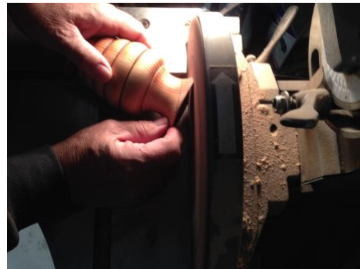
Figure 17. Start shaping top on a flat sander.
