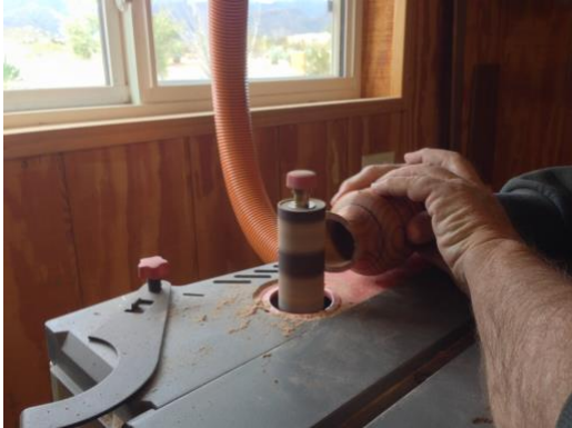
Figure 19. Shaping the final top curves.
