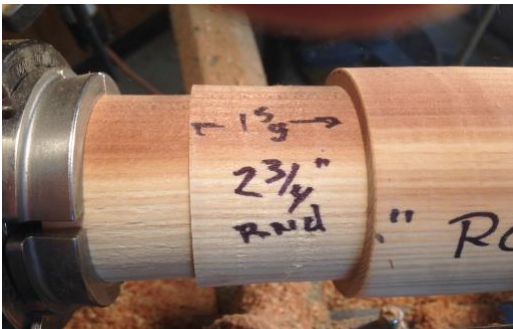
Figure 6 After turning both tenons mount the blank in a chuck and turn the top of the vase (2-3/4" in my case).
