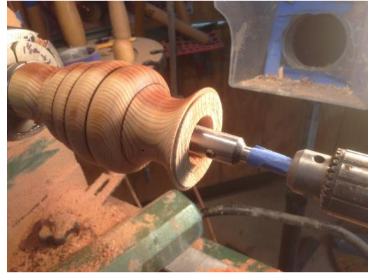
Figure 11. Part off the top Tenon and establish the depth of the vase. Then drill to the desired inside depth. If you use a forstner bit, be sure to drill at slow speed clearing the chips often so that the bit does not become trapped.
