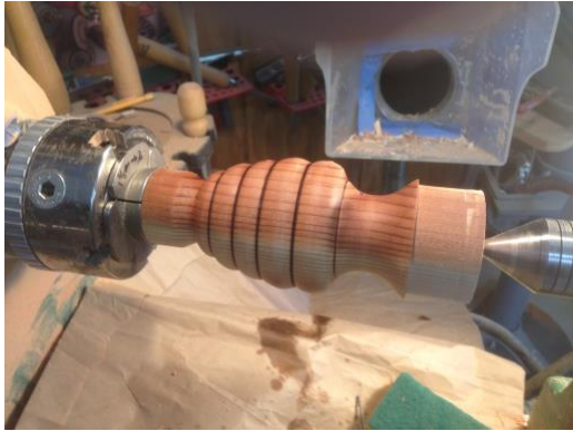
Figure 10. Reverse chuck the blank using the tail stock to seat the blank prior to tightening the chuck.
