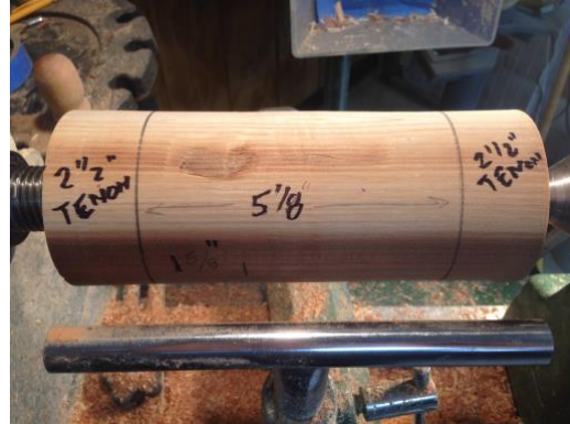
Figure 5. Round the blank to 3-3/4" and mark off the tenons leaving 5-1/8" for the final piece.
