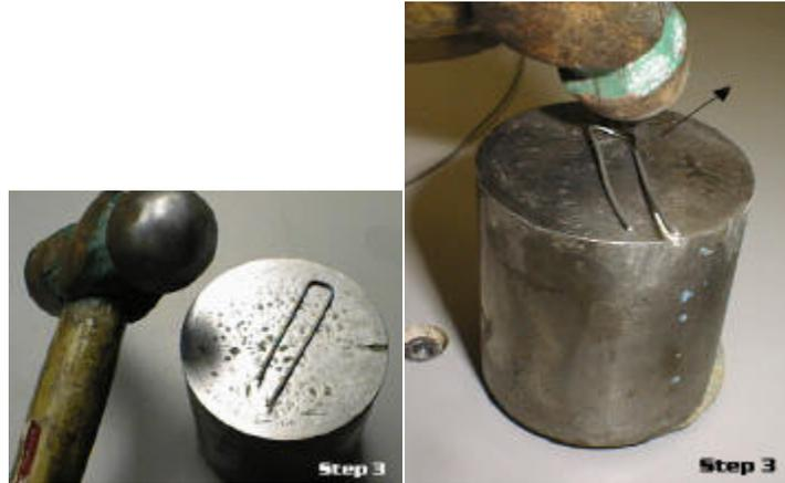
Shaping of the tip is done by hammering the wire flat using a steel slug and a small ball peen hammer. This is a technique that will require a little practice. You will need to stretch the metal in both corners outward to form the scale shape, this is done by hammering at an angle dragging the metal out. Work slowly and hammer lightly, the wire will flatten easily. It will take a tip or two to get the hang of this, but once learned is easily repeated.
