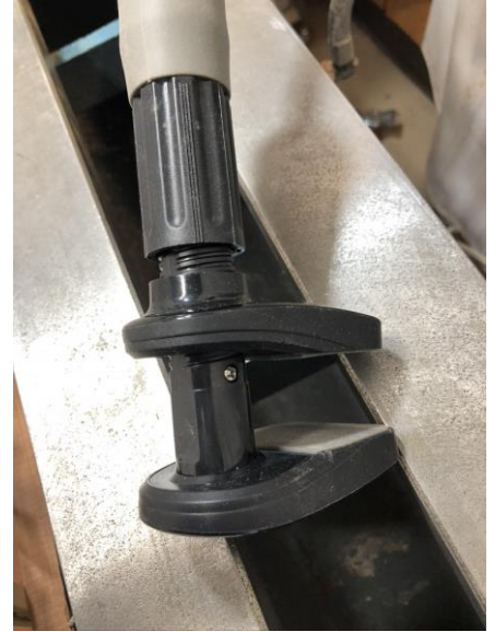
Top screw clamp facilitates easy lathe bed clamping
